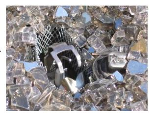
Burner Assembly with a 'fence' around it. We created this fence using a galvanized steel screen material we buy in the roofing section in Home Depot. Make sure that when you install the fireglass that none of it falls inside the 'fence' you have created around the Pilot Burner. In the end, you should still be able to see the Pilot Burner as shown in this photo.
