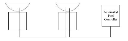
Note: In the picture at left, there is only one conduit but there are 2 pairs of wires. One pair of wires goes to the first bowl, the second pair of wires continues onto the second bowl.
